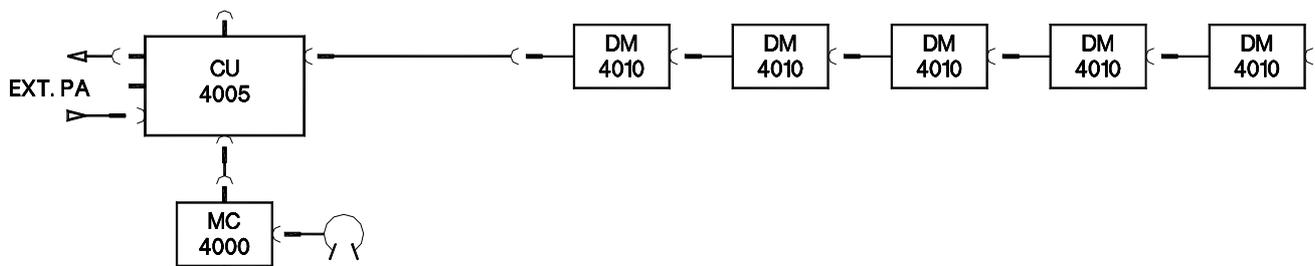
In this situation the level of the DM/CM4000 units connected to the Delegate Microphones connector is adjusted with the Microphone Volume control,
