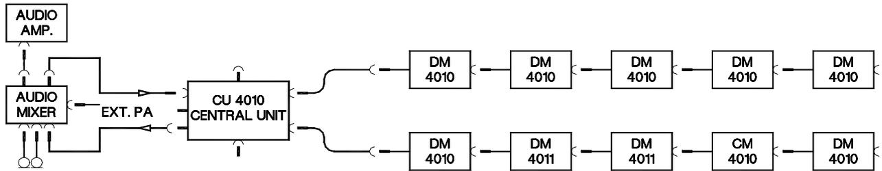
In this set-up an external PA system is connected along with some auxiliary microphones. Since only one input connector is available on the CU4005 /CU4010 unit, it will be necessary to make use of an external mixer.
