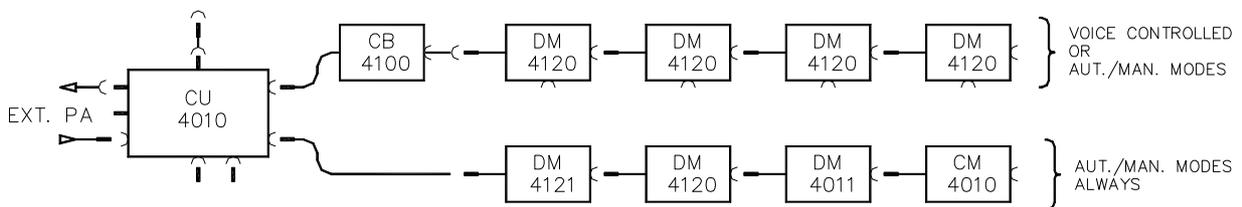
The CB 4100 Control Box should always be present in a set-up when voice activated
