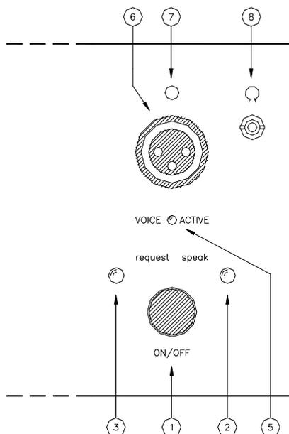
The additional connectors and lamps on the DM 4100:
