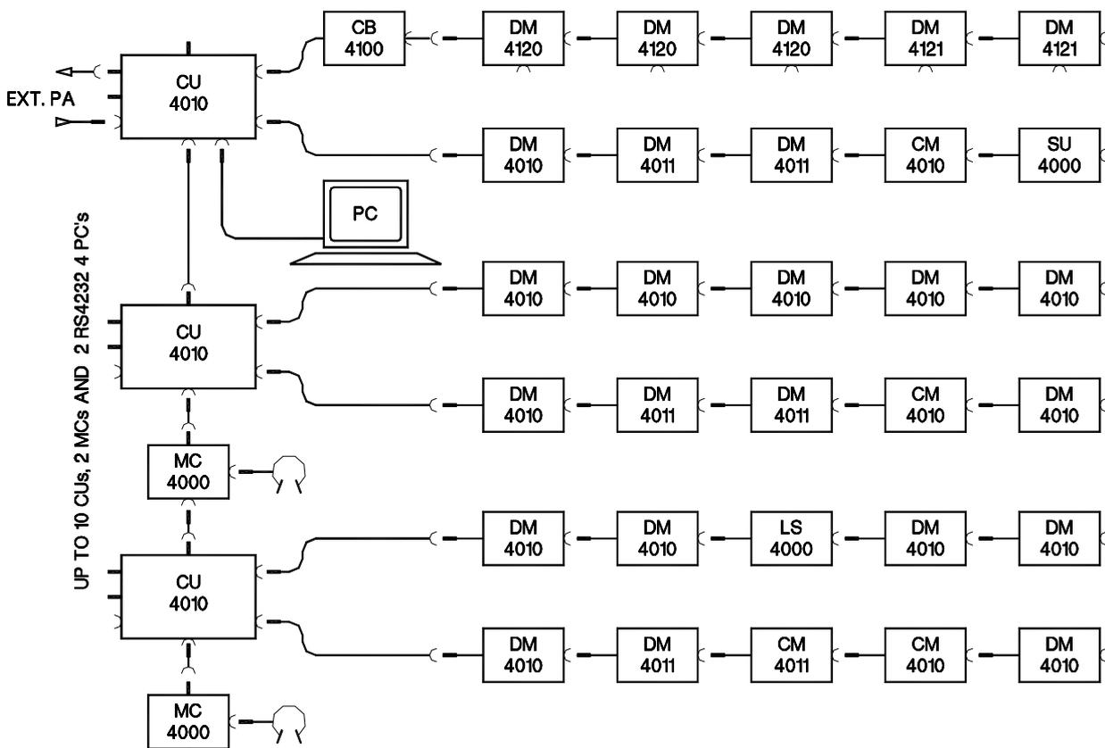
The central units are interconnected with the control link cables in the D9-connectors NEXT CU4005/CU4010 and PREVIOUS CU4005/CU4010.
