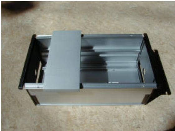
Place the spacer rail over the profile close to the holes (as shown on the photo), which are going to be pilot-drilled. Use a 1,5 mm drill as close to the centre of the holes in the profile as possible. Screw in the two screws. Move the spacer rail to the next holes, pilot-drill and screw in these screws.
