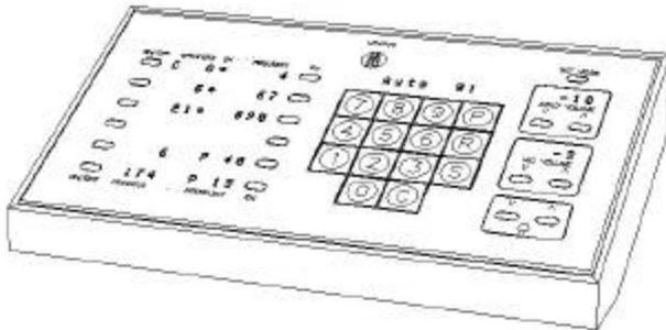
The MC4000 Microphone Control is a compact desktop switchboard designed for the CDS 4000 system. It is used as an operating switchboard to control the connected Delegate/Chairman units.
