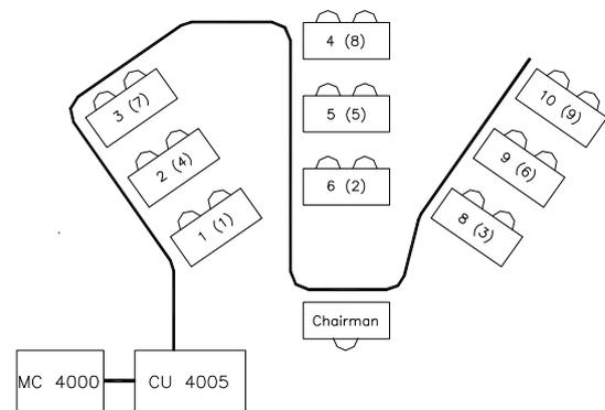
The connection between physical and logical numbers is established in the programming mode by the operator and preserved during power off. The programming described here will normally only have to be done once upon installation of a permanent microphone system. If more than one MC4000 panel is used, it is possible for the two MC4000 panels to operate with independent conversion tables (this is not recommended).
